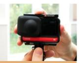
In its protective case, the camera can screw onto the top of the stand. Make sure the camera is level (not at an angle).
